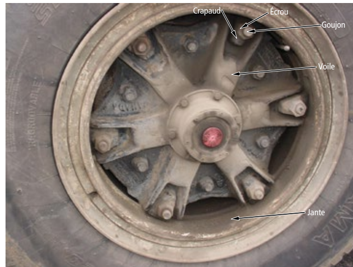
FIGURE 45 | Roue moulée ( spoke wheel )
