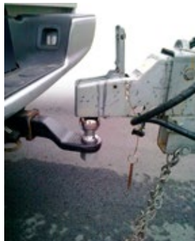
FIGURE 5 | Main et boule
