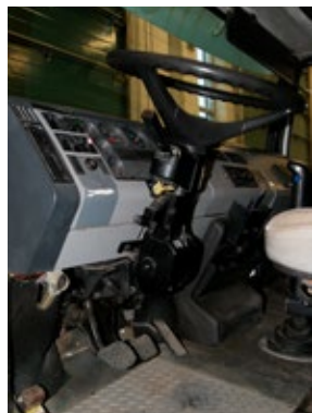
FIGURE 25 | Colonne de direction
