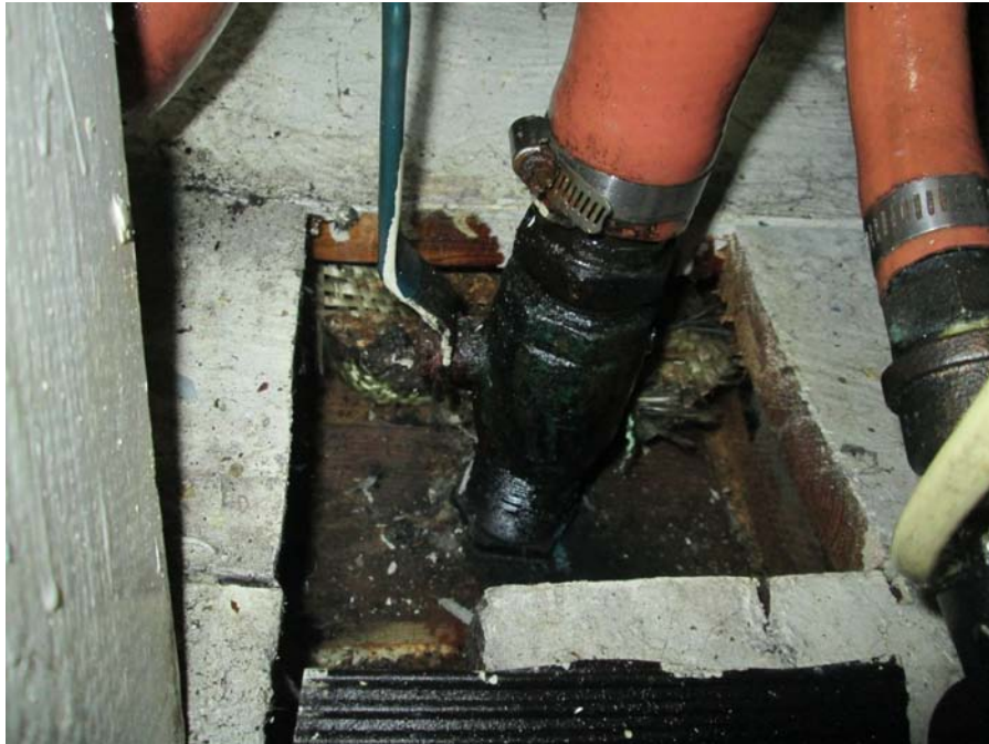
Photograph 21 - Toilet discharge hull connection
