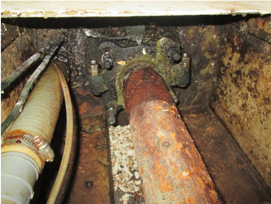
Photograph 27 - Shaft penetration at aft engine room bulkhead
