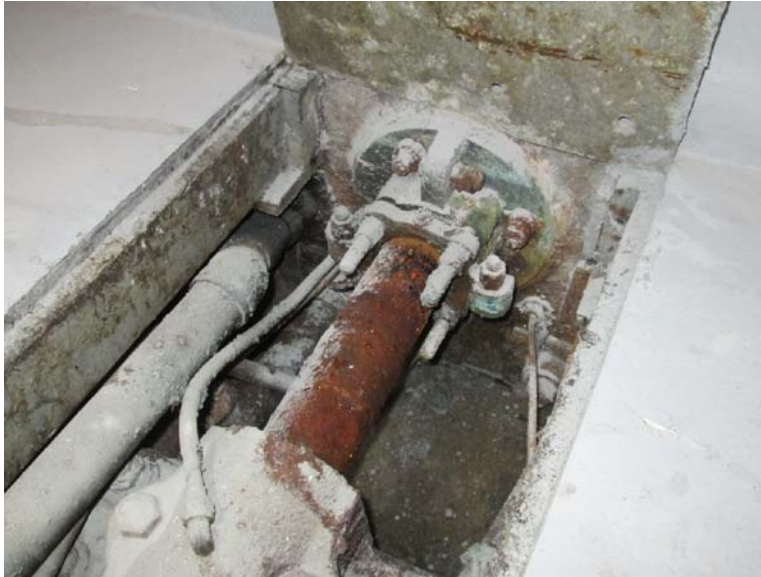
Photograph 25 - Shaft seal at forward fish hold bulkhead
