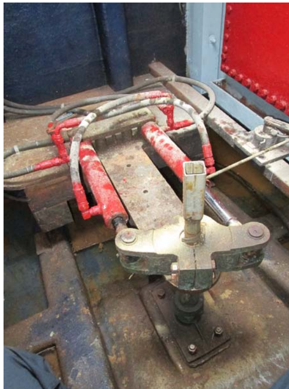
Photograph 12 - Steering Gear
