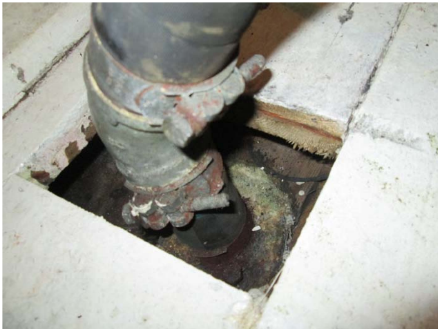
Photograph 20 - Keel cooler hull connection (typical)
