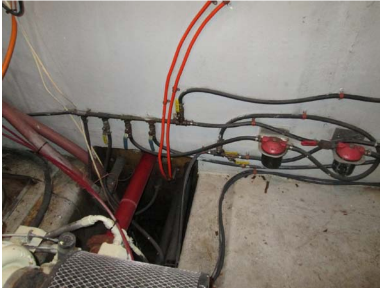
Photograph 17 - Fuel manifold and filters
