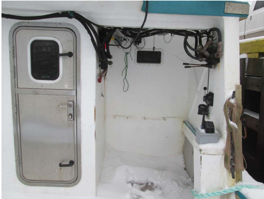
Photograph 11 - Deck equipment hydraulic controls
