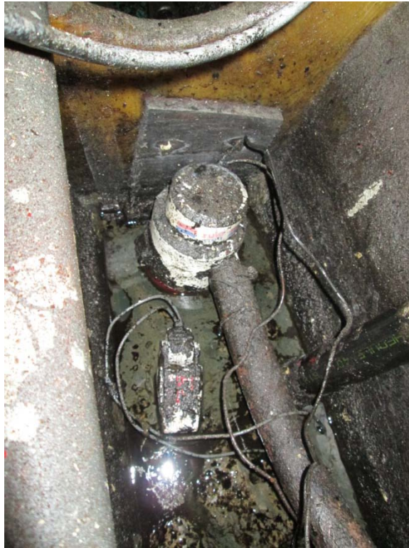
Photograph 19 - Rule bilge pump and switch, engine room aft
